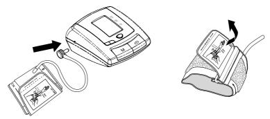
Put your left arm through the cuff loop. The "OK" range indication should be positioned closer to yourself with the rubber tube pointing in the direction of your arm. Position the artery mark (Φ) over the main arteries (on the inside of your arm) in the upper arm.
